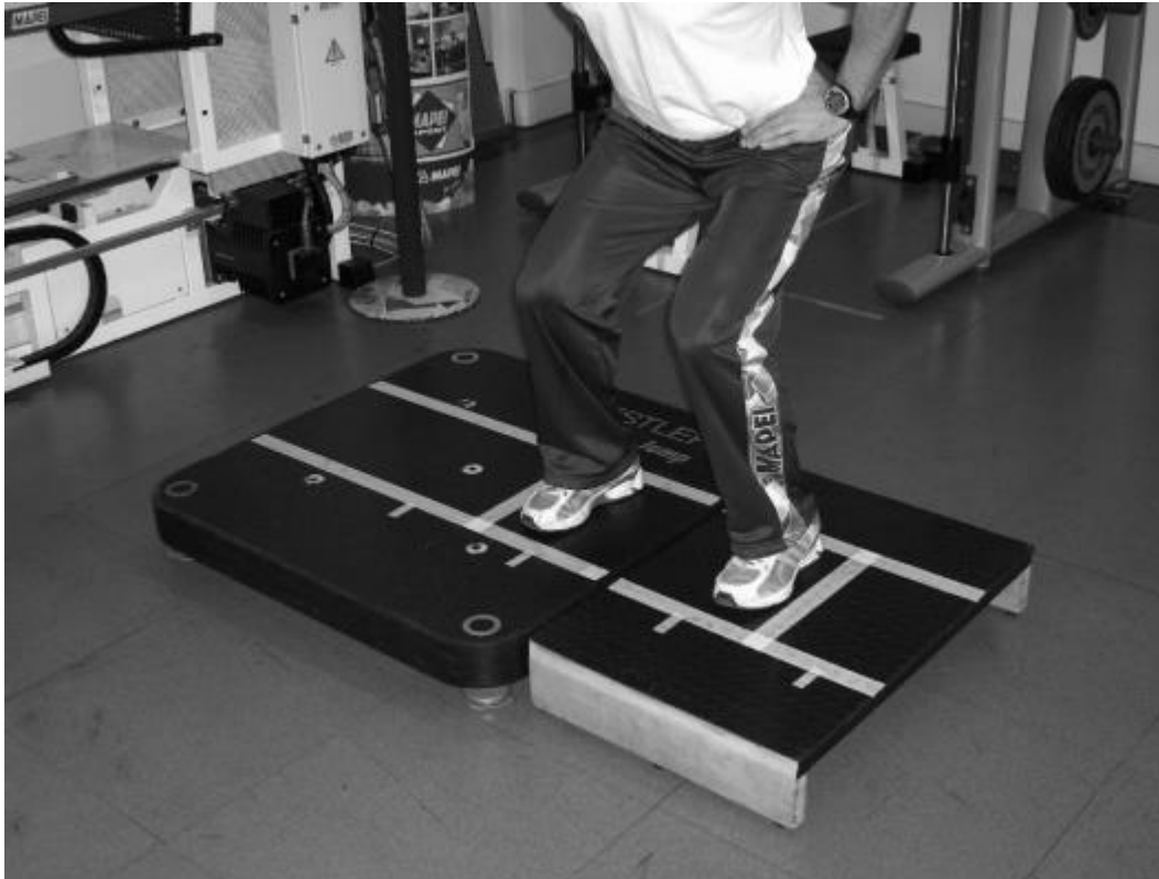
Figure 1: DL-CMJ test performed with single force platforms. One leg on a force platform (right leg) and one leg on wooden “dummy” platform (left leg).
