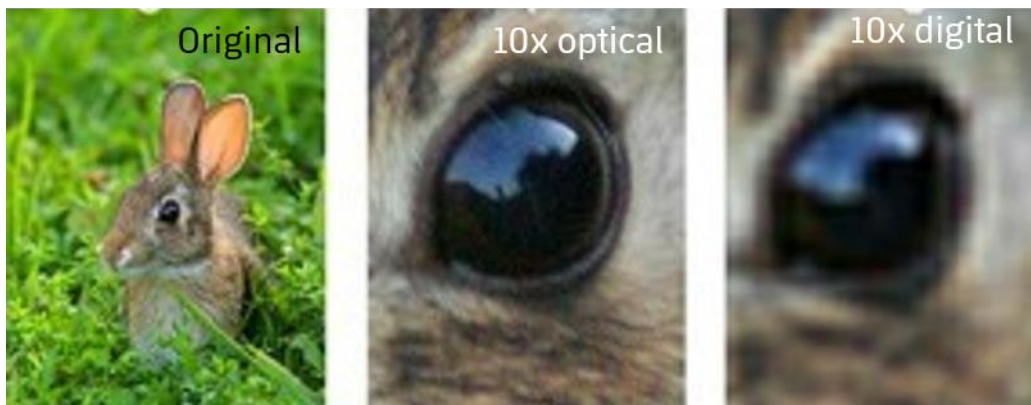
Figure 13: Comparison between optical zoom and digital zoom
