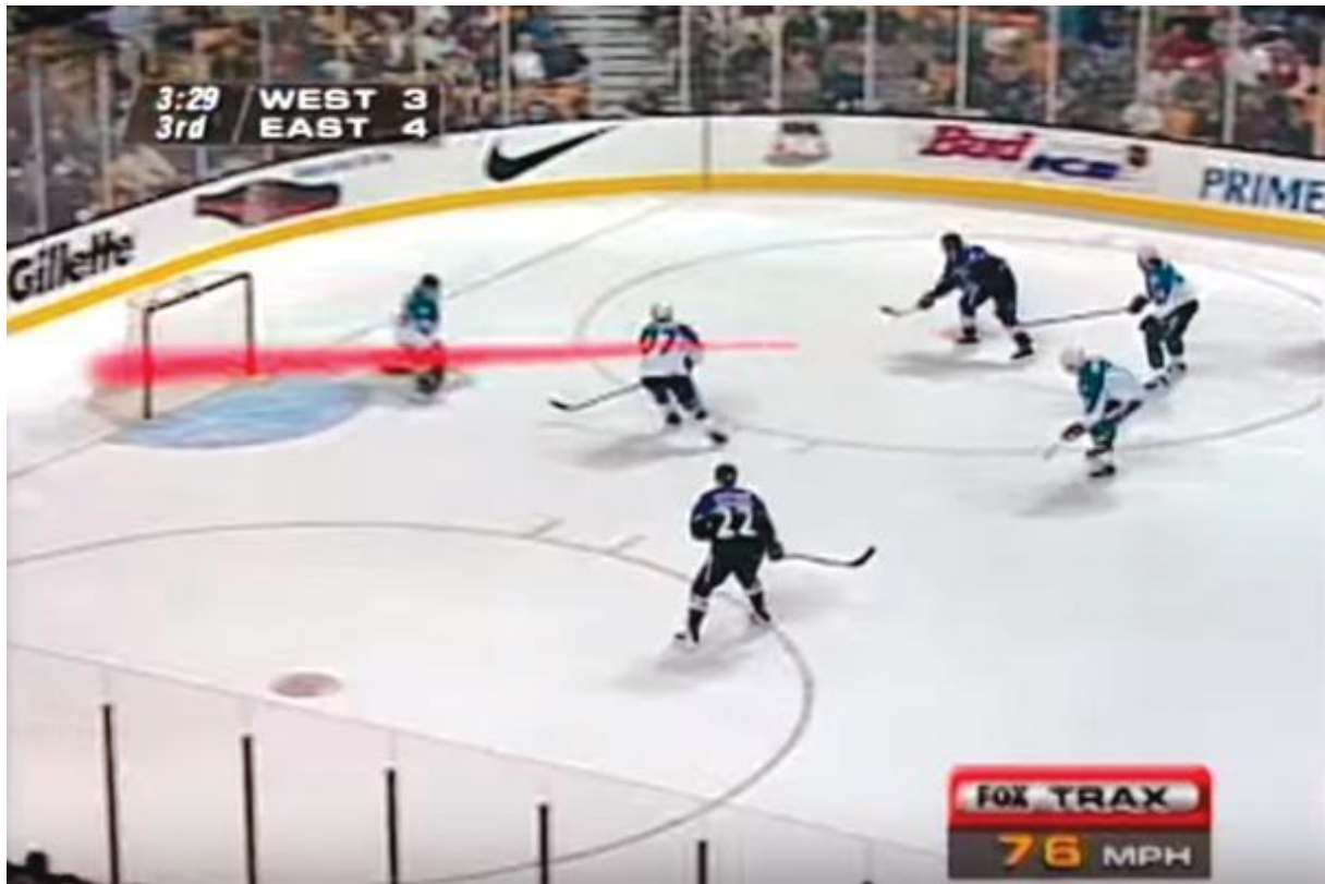
Figure 2. FoxTrax - the glowing puck
