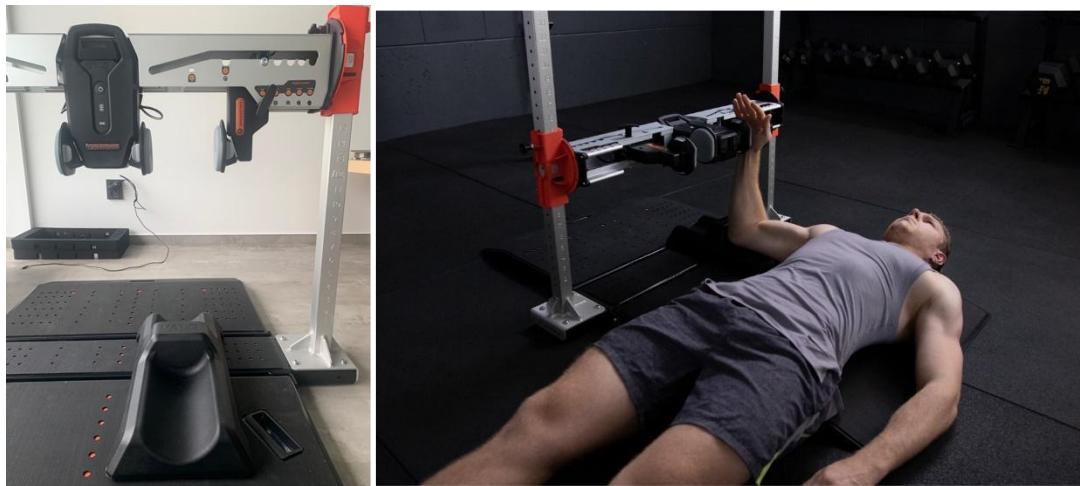
Figure 6: Force Frame Isometric Shoulder test with moulded elbow support
