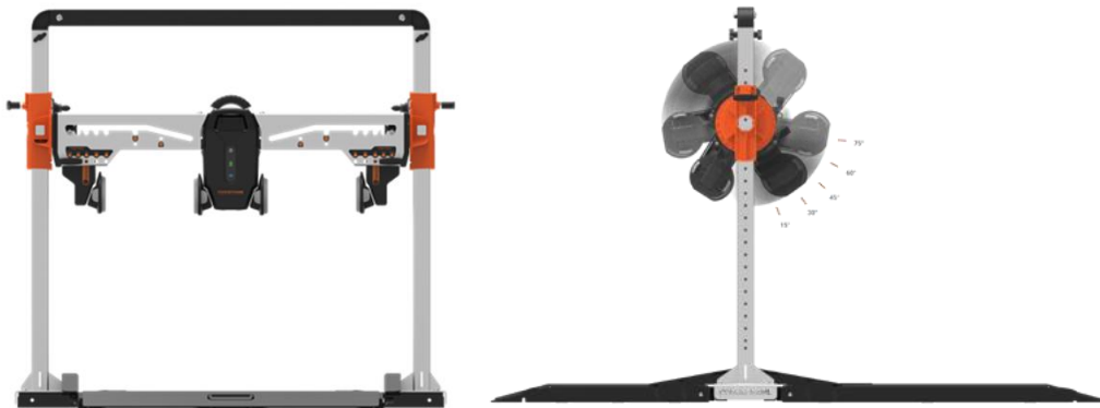
Figure 9: The force frame and positions for assessment of internal and external rotation strength
