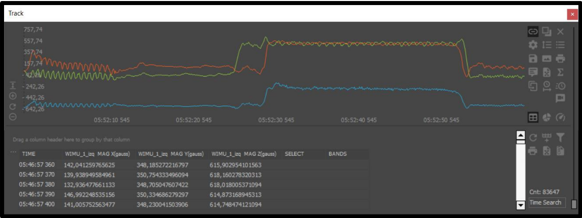
Figure 28: Magnetometer sensor and its three channels
