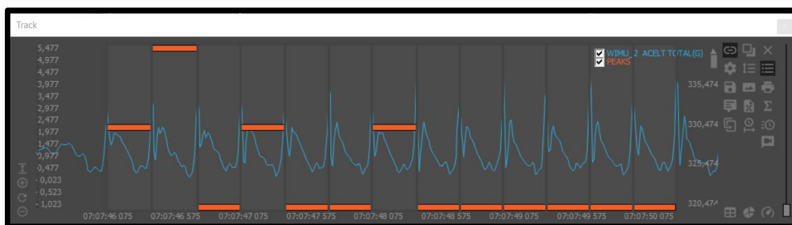
Figure 14: Application of an algorithm to detect supports
