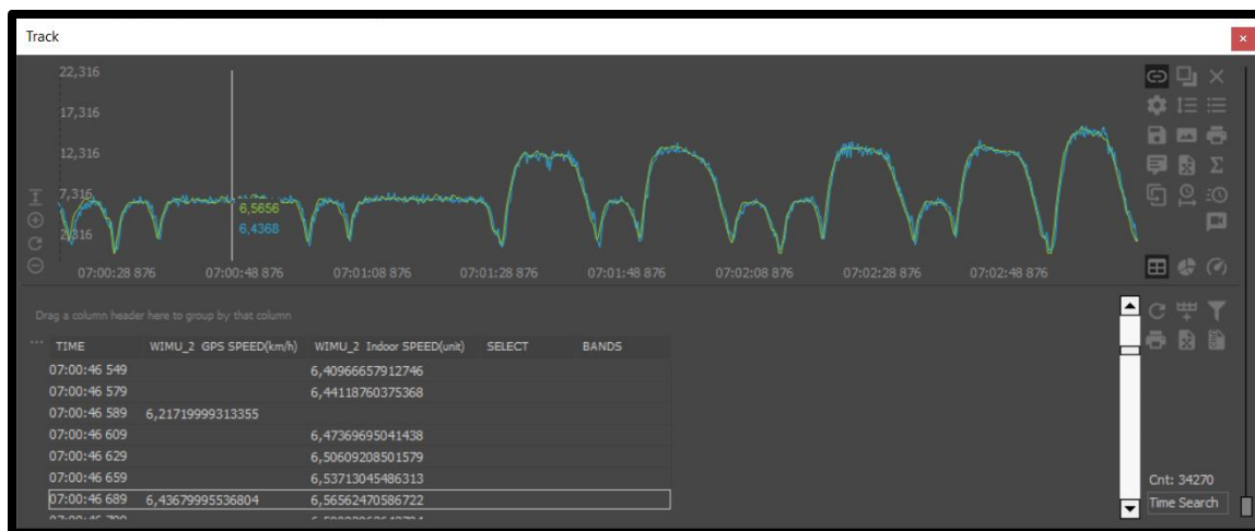
Figure 8: Speed measured with GNSS/LPS technologies
